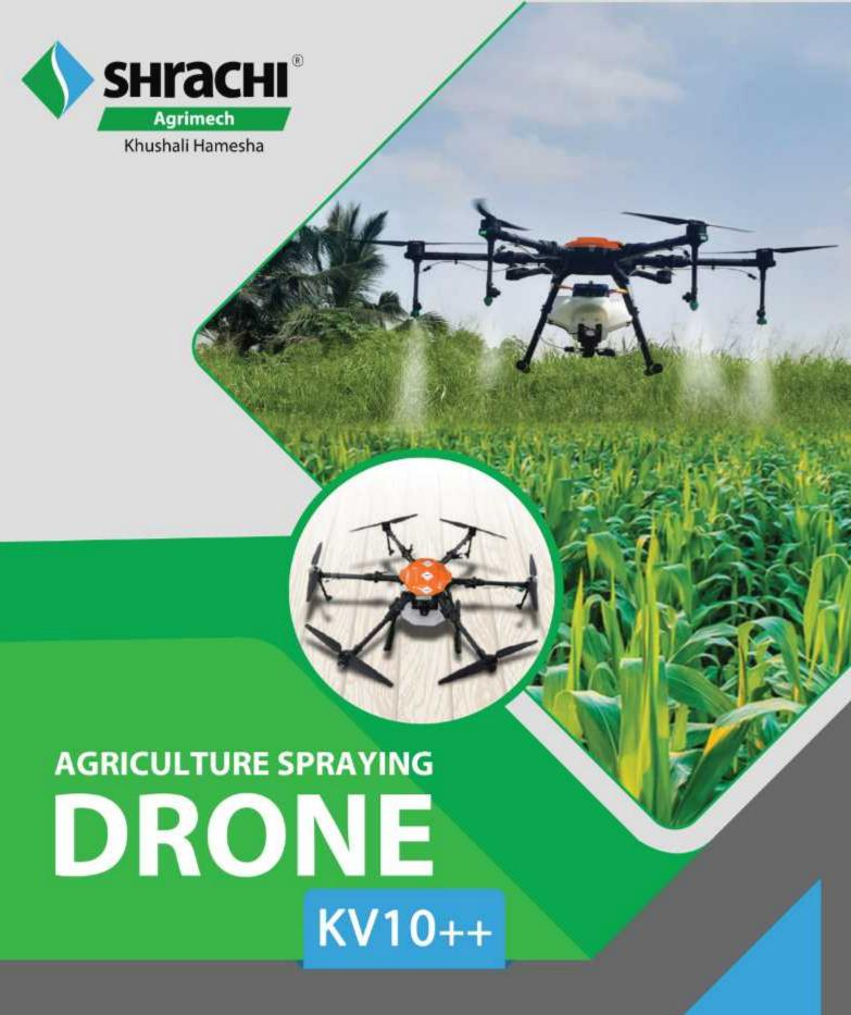
KV10++ series agriculture drone is a Hexacopter drone manufactured with high strength carbon fibers, impact-resistant molded materials and aerospace grade aluminium materials.
